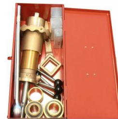
32mm and 50mm Tappings. Major Tap Machine 1. Ratchet 2. Adapter 3. Jumper valve 4. Feed handle 5. Drill 6. Barrel 7. Valve key 8. Drill body 9. Cap or bonnet
