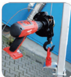
Fixed at the tripod, using an adapter plat with stop ring
